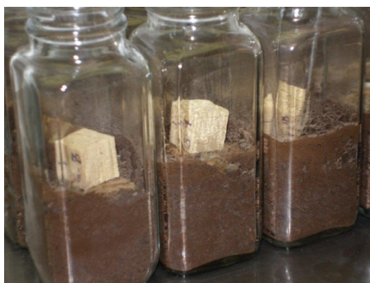
Fig. 2 – Experimental set up for wood decay test of sterile untreated blocks on top of fungi inoculum and feeder strip in soils jars for brown rot fungi.
